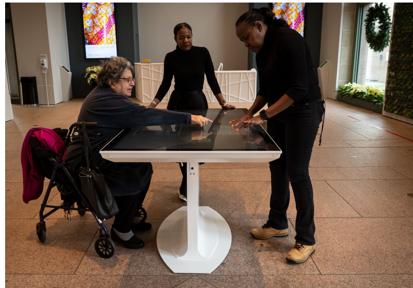
Visitors can roll up and under a 65" Ideum touch table at the Smithsonian National Museum of African Art. At this exhibit, content is presented along all four sides. Under the "strict" interpretation, the reach here would be 16.3" (414 mm).
