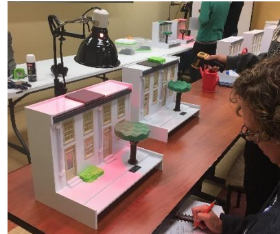
Heat lamp simulates effects of high heat on building materials
