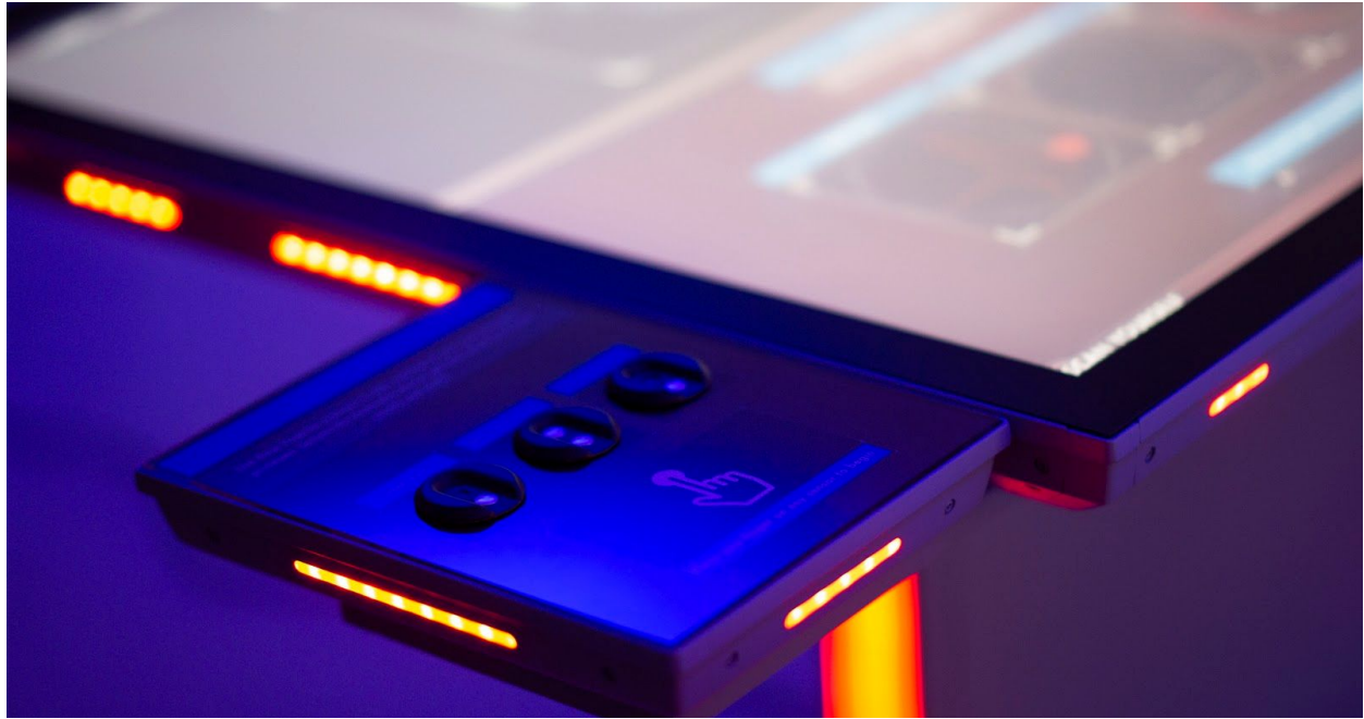
Figure 2: Fingertip sensor panel for Scan Yourself module. The panel extends to the left of the module.
