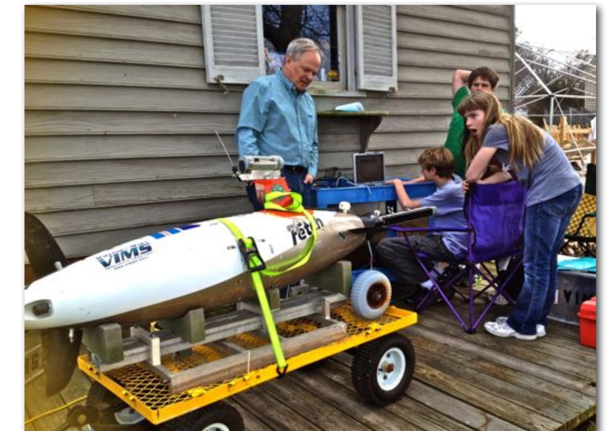
Having installed the sonar and GPS, students conduct a pre-launch test of the free-swimming AUV
